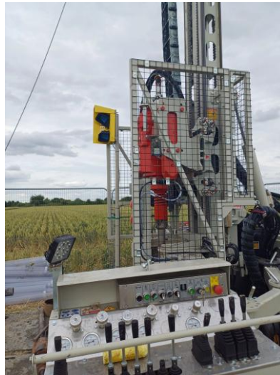
Figure 3. Image showing SAFER G 2025 Series Sensors mounted on side guards
